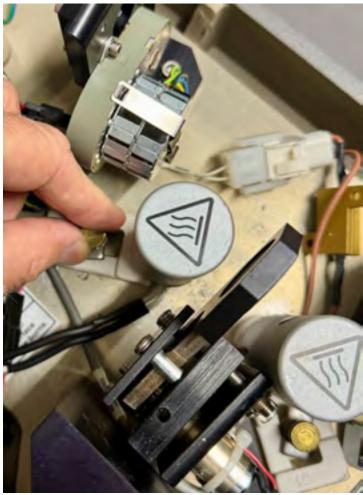
The brass knurled screw is not removed (just loosened) so the small flat rectangular plate can be rotated and allow to remove/install the source.
